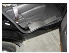
**STEP 2**Remove the passengers side rear door sill.
